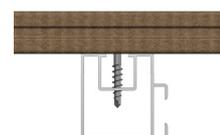
Once the first terrace part has been installed, you simply place the clamps on the profile. Make sure that the long end of the hammerhead nut is positioned along the direction of length of the aluminium girders.
